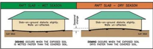
Exaggerated, seasonal-changing surface shape of soil under small buildings for both framed and slab on ground floors.
